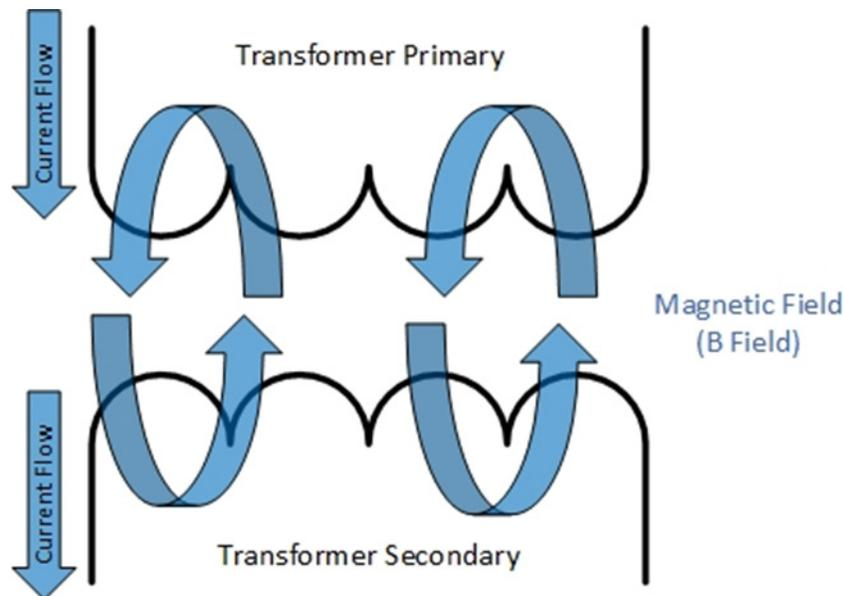
This "transformer action" is further intensified as the amount of parallelism between a pipeline and the electrical conductors increases and can result in significant induced voltages and currents on the pipeline. These induced effects can be a danger to personnel but also have the potential to damage the pipeline coating and lead to AC corrosion effects on the structure or pipe.
