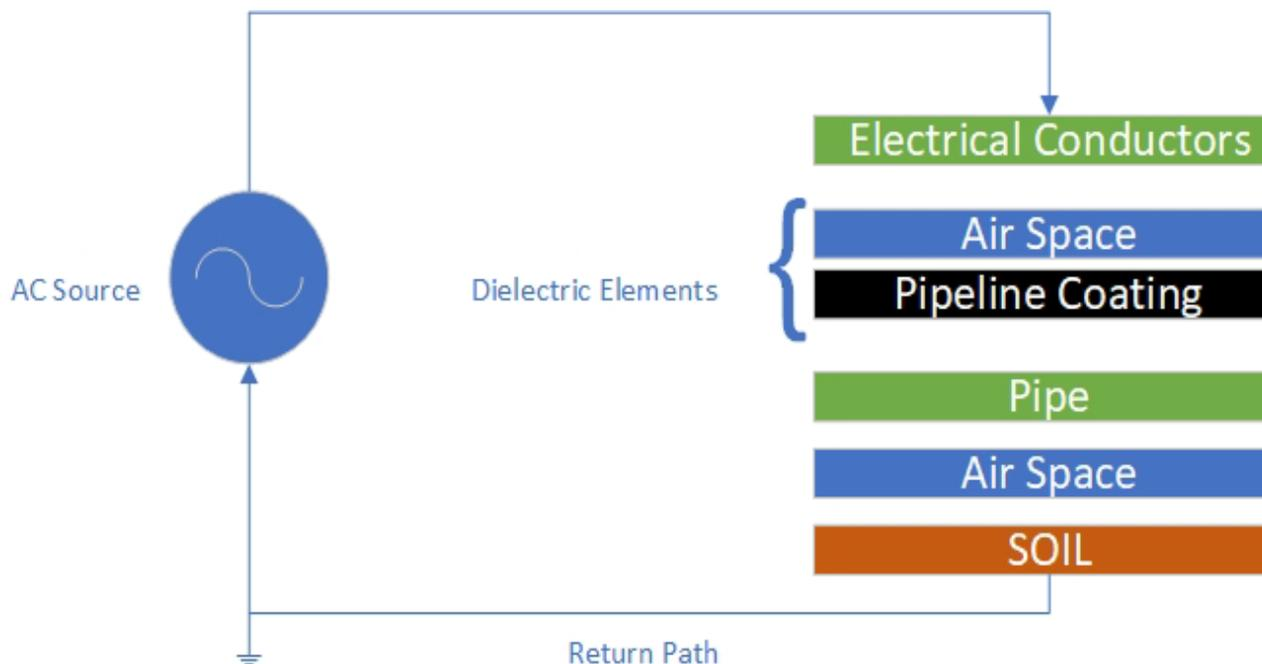
It should be noted that the interaction between the dielectric elements is much more complex than is represented in the above diagram. As an example, any additional elements present will change the relative permeability (dielectric constant) between the conductors, but it also may act as a return path back to the voltage source, creating multiple series capacitances that must be considered.
