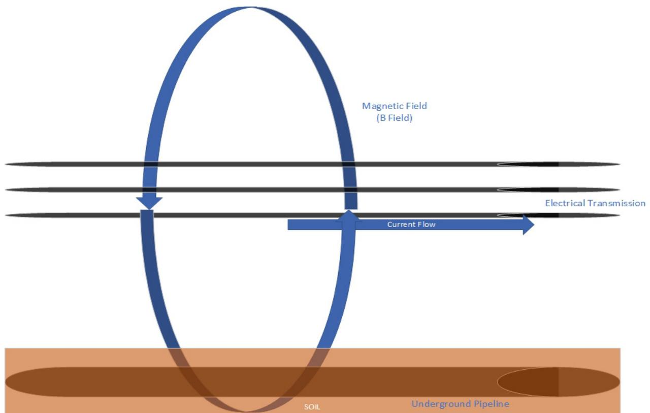
Another way to consider the inductive coupling described above where voltages and currents are induced electromagnetically onto a pipeline is to recognize that this is the same "transformer action" in which the primary winding of a transformer induces current flow through secondary windings.
