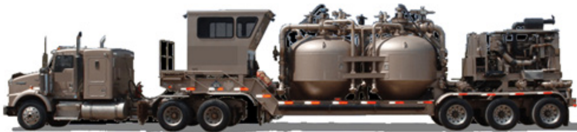
Typical Nitrogen Pumper Truck
